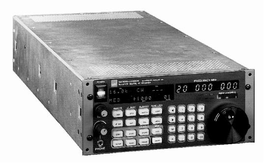
The WJ-8712P is a fully synthesized, general-purpose HF receiver for surveillance and monitoring of RF communications from 5 kHz to 30 MHz with 1-Hz tuning resolution. The unit is packaged in a 3.5 x 8.25 x 20 inch (8.89 x 20.96 x 50.80 cm) half-rack enclosure, and utilizes the same RF and Digital printed circuit boards as the WJ-8711A. By combining analog and digital signal processing, the WJ-8712P achieves high performance at low cost.
